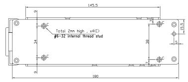
Measuring the screw protrusion first:
