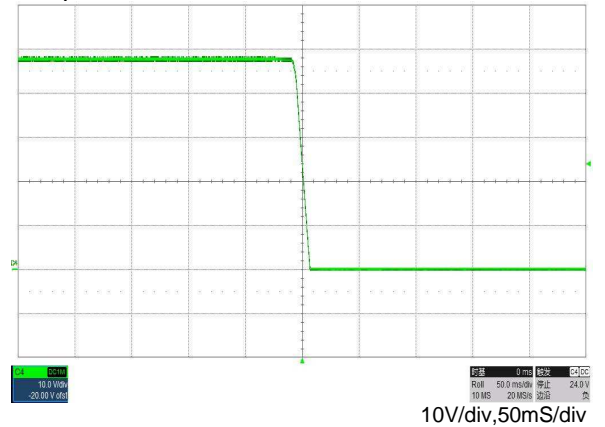
Output turn-off rated load
