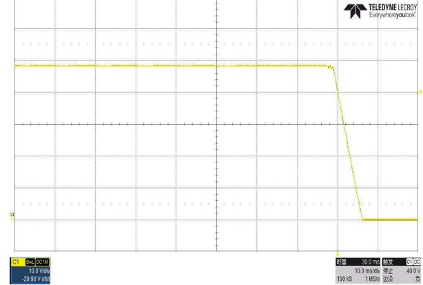
Output turn-off rated load
